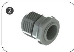
Cable Gland · M20 fits Cable O.D. 10~14mm · M25 fits Cable O.D. 13~18mm
